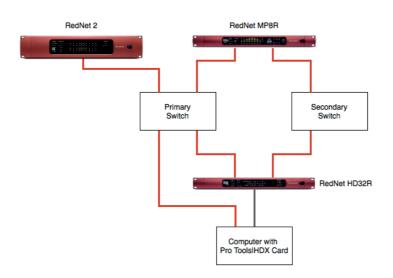
RedNet units with only one network port must be connected to the Primary Switch Only.
